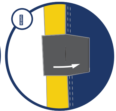
8 ATTACH THE CORNERS OF THE CABIN TO THE 4 POLES WITH THE VELCRO STRIPS
