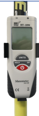
HZ-24 : Differential pressure gauge
